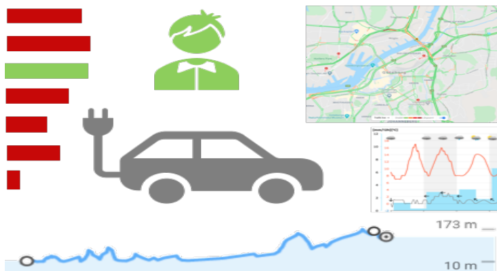
Figure 6 - Information sources for a smart BMS predict range for an electric vehicle
